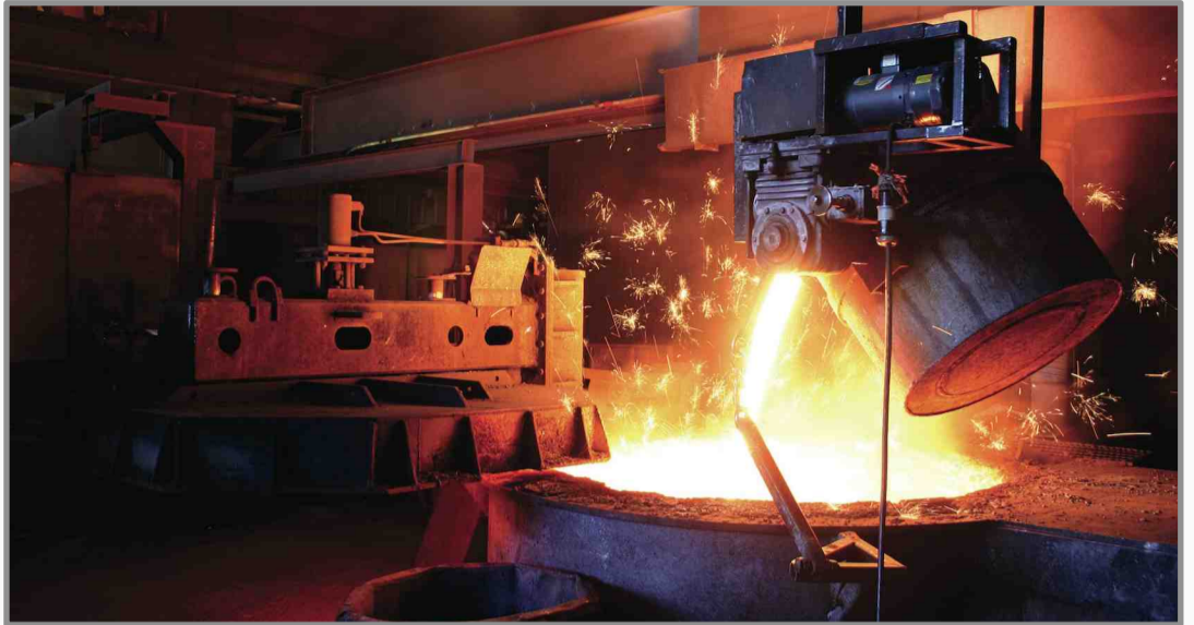
Fuelling the fire: A transfer ladle hot-charges Leth Iron's 40,000lb capacity Ajax furnace
