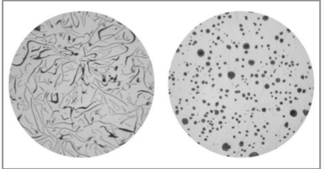
Microstructure of cast iron (left) and ductile iron (right) under 100x magnification
